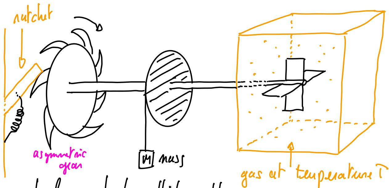
Idea: The gas molecules randomly collide with the paws, which promotes clockwise (cw) & counter clockwise (ccw) rotations of the axis.
