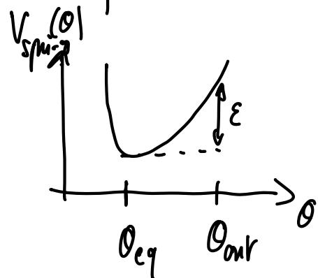
This requires an increase of energy of the spring, which is then dissipated once the wheel has rotated  $\Rightarrow$  heats up the spring.
